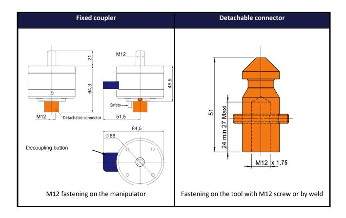
Safety: To avoid a decoupling by accident, the button cannot be pushed if the load is not laid on a support.
